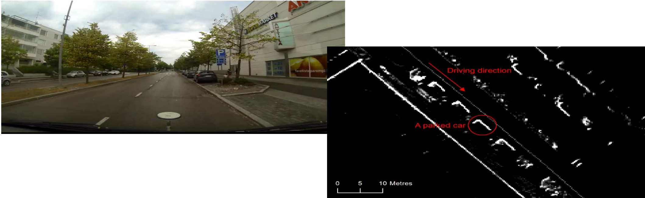
Figure. a) Part of the street Espoonlahdenkatu as recorded on the reference video during data acquisition Drive 1. b) Raster representation of the car-based laser scanner data. The pixel value of each 0.3 \text{ m} \times 0.3 \text{ m} cell corresponds to the number of laser points inside the cell. Parked cars appear as L shaped clusters of bright pixels.
